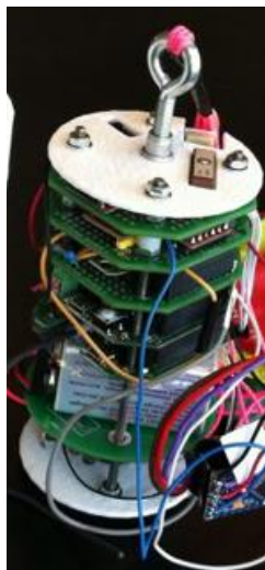
Fig. II: Structural design of our CanSat.
