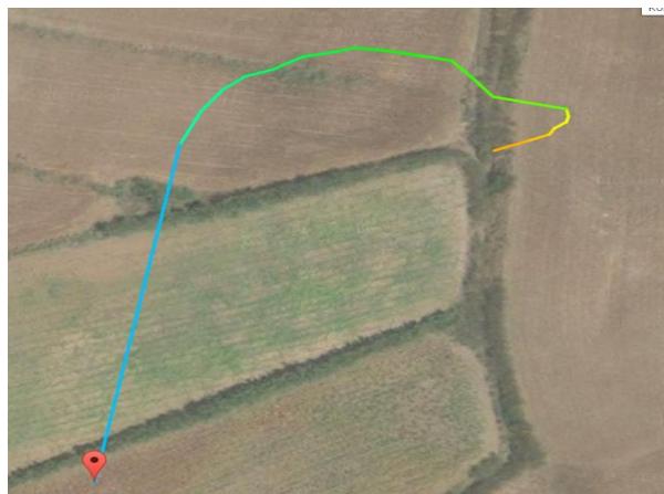
Fig. XVI: Tracking of CanSat by using GPS. Colour indicates the altitude of the CanSat.
