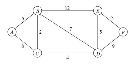
Find the shortest path from A to F in the above network, by letter indication. (Diagram is not to scale)
