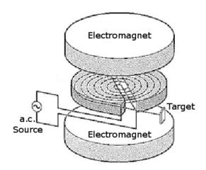
Cyclotrons are located in the same hospital as the PET scanners and are used to manufacture radioactive nuclei. Cyclotrons are circular devices in which charged particles are accelerated in a spiral path within a vacuum. The particles are accelerated by a rapidly alternating voltage and acquire high kinetic energies. They spiral outwards under the influence of the magnetic field until they have sufficent velocity and are deflected into a target producing radioactive nuclei, including carbon-11.
