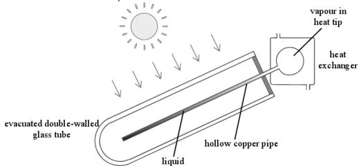
In a vacuum-tube collector, each tube consists of an evacuated double-walled silvered
