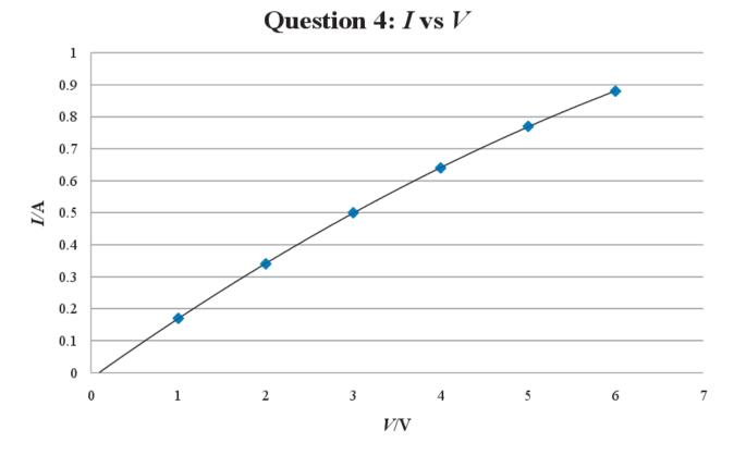
4. A student was asked to investigate the variation of current with potential difference for a thin metallic conductor. The student set up a circuit using appropriate equipment. The student recorded the values of the current *I* passing through the conductor for the corresponding values of potential difference *V*. The recorded data are shown in the table.
