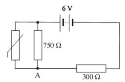
In the circuit diagram, the resistance of the thermistor at room temperature is 500  $\Omega$ . At room temperature, calculate
