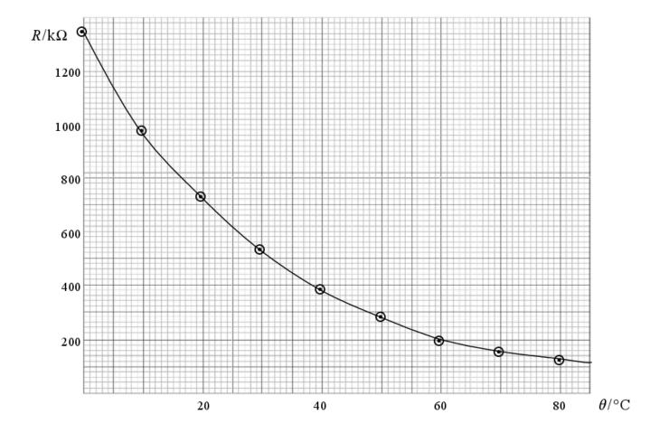
The thermistor is used in a circuit to keep the water in a tank at a constant temperature. What is the temperature of the water when the resistance of the thermistor is  $420 \text{ k}\Omega$ ? (6)
