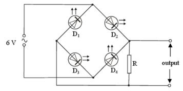
The circuit shows four light-emitting diodes connected to a resistor R and a 6 V a.c. supply of frequency 1 Hz.
