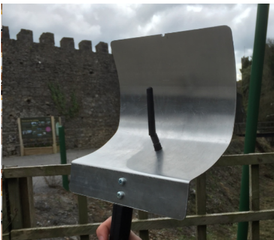
Left: Semi parabolic reflecting dish used in National Final
