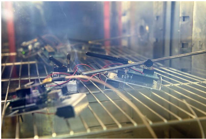
Arduinos inside Industrial Temperature Regulator
