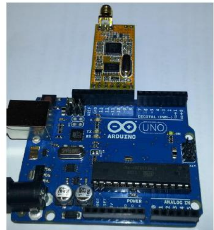
Figure 13. Connecting the transceiver to the Arduino UNO
