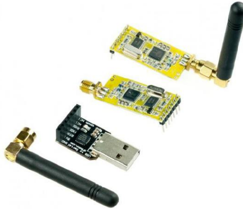
Figure 10: The APC220 communication module (from www.DFRobot.com )
