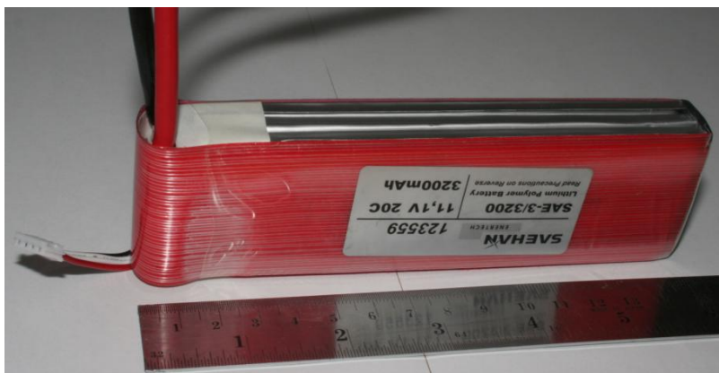
Figure 33: A lithium polymer battery, which is rechargeable with special balanced-charging equipment. (source Wikimedia.org)
