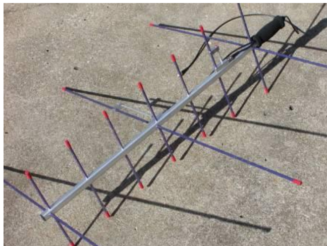
Figure 37: An "Arrow" which is a Yagi antenna for operation at 2 different frequencies
