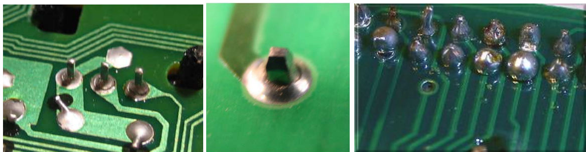
Figure 30: photographs of bad soldering (courtesy of T-Minus)
