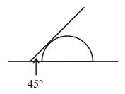
The rod is in equilibrium inclined at  $45^{\circ}$  to the horizontal. The hemisphere, of radius 1 m and weight 40 N, is in limiting equilibrium (that is, just on the point of slipping).
